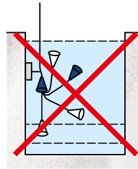
Image 6. Avoid fixing the float such that a sharp corner can cause kinks or wear to the cable.
